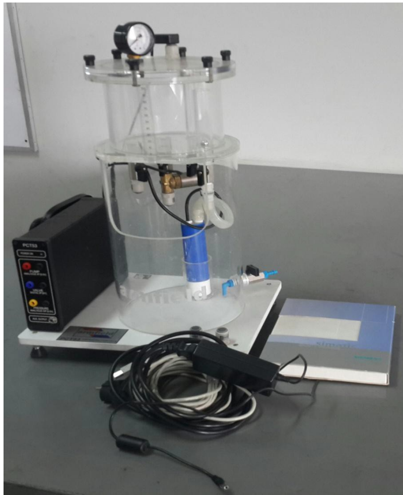
Fig. 7.9: PID Pressure Control Device
